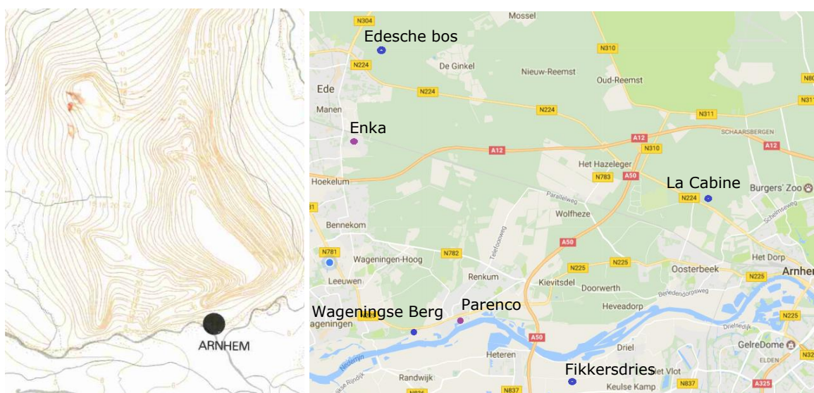
Figure 5.6 A) Isohypses (groundwater contour lines) in the Veluwe region and sandr area, and B) location drinking water pumping stations and large industrial abstractions
